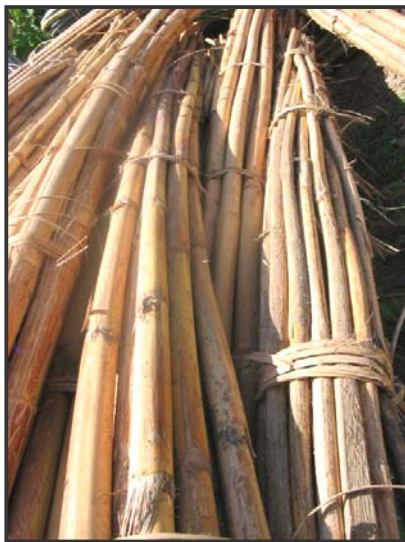
Figure 2.3. Scratched surface of large canes caused by dragging in transportation
